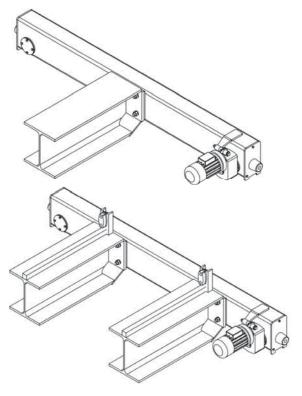
Main girder, side joint, standard, profile, cut bottom corner for single and double girder bridge crane
