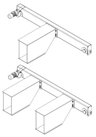
Main girder, side connection, standard, box, cut bottom corner for single and double girder bridge crane
