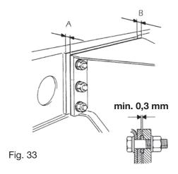
The dimensions A and B (shown in fig 33) may be different from each other; this difference does not affect the alignment between the wheel axles of the heads and the orthogonality between the heads themselves and the beams, which is determined by the machining of the alignment bush seats.
