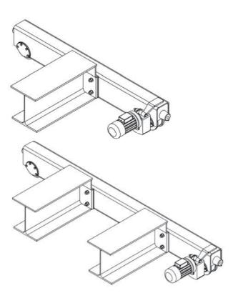
Main girder, side connection, standard, profile, rised corner for single and double girder bridge crane
