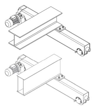
Main girder, bottom joint, standard, profile, for single suspended girder bridge crane.
