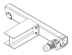
Main girder, side joint, standard, profile, for single girder bridge crane
