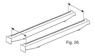
• Wheelbase can be verified directly on the hoist trolley or on the technical documentation.
