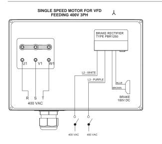
Separated brake feeding 400VAC monophase Brake 180V DC
